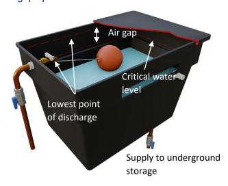
In the case of wholesome water applications, the overflow should be fitted with a screen and light cowl
